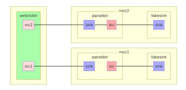
webrtcbin exposes one src pad per simulcast stream / ssrc
