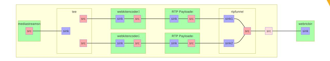
rtpfunnel aggregates encoded/payloaded streams and sends the merged stream to webrtcbin
