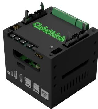
Hardware: *Host PC, serial, CAN emulator, USB Switch + Hub, Bluetooth/WiFi, HID emulation, ...*
