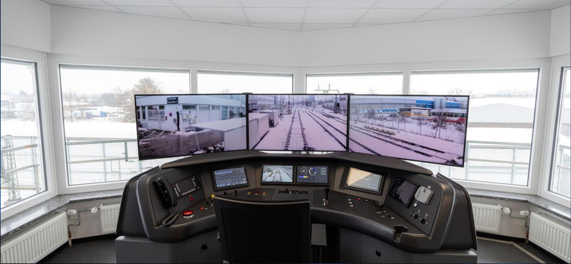
Driver's desk in the Remote Operation Centre. Copyright: Deutsche Bahn AG / Thomas Kiewning
