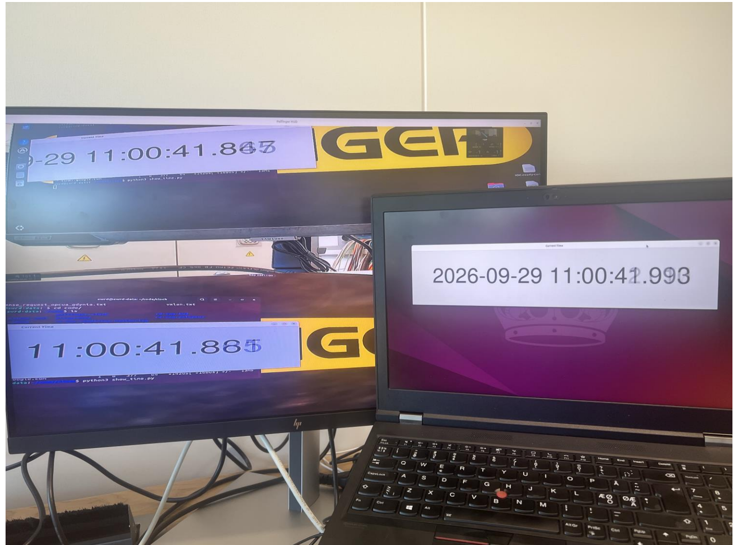
Glass to glass method: remote location display in Poland (left) and on-site display in Norway (right)
